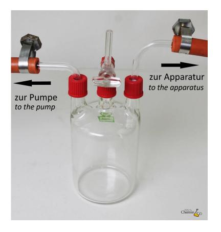
The two outer openings are connected to the apparature and the pump. The tubes should always be secured with tube clips.
